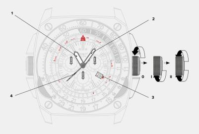
Hour hand Working position Minute hand Date setting position Time setting position Date display Small seconds hand
